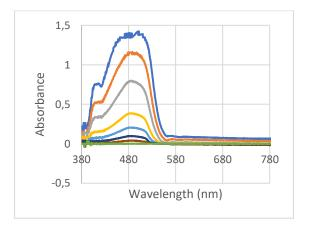
The absorbance is obtained from  $I_0$ , which is the intensity showing on the spectrometer at 480 nm on a blank solution (when no pigment is present, for instance a cuvette with distilled water only), and I, the intensity measured by the spectrometer at 480 nm for a given solution at a known concentration.
