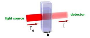
Absorbance is measured by comparing the intensity of the beam of light entering the
